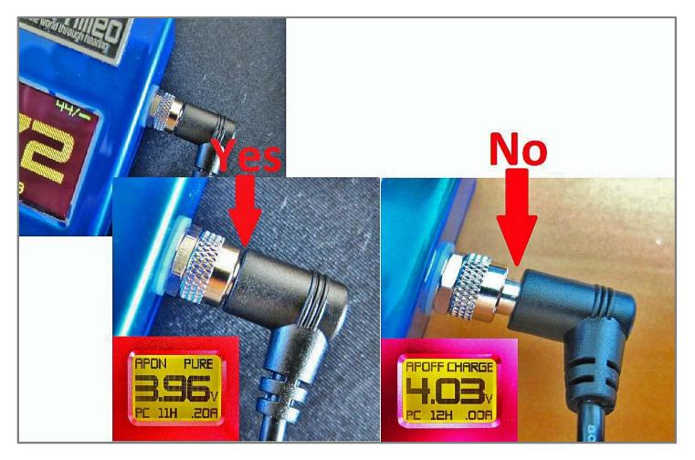
Figure 3 Insert the power cable into the Audiophilleo, then **GENTLY** screw it on, then push it fully in. **Note that** with newer units it is only necessary to gently thread the cable in. After that it is already fully pushed in.
