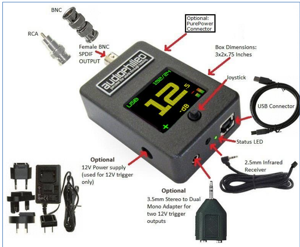
Figure 1. Connections (Items not to scale)
